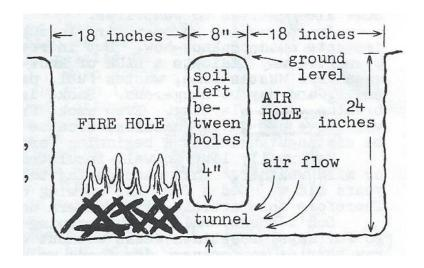
Build your fire in the bottom of one hole. Regulate the air flow by partly covering outer-hole. CAUTION: this fire can burn hot enough to ruin a pot. Tim Leathers, TN, May & Dec.
