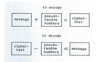
This program encodes letters, numbers, & punctuation marks. Here's a sample coded message to show you what the ciphertext looks like:
